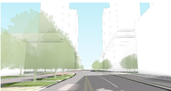
New Cherry Street looking south just after crossing the new bridge and landing on the island shows a wider right-of-way to allow room for multi-modal travel onto and off of the island, including 2 vehicle lanes, separated bi-directional
