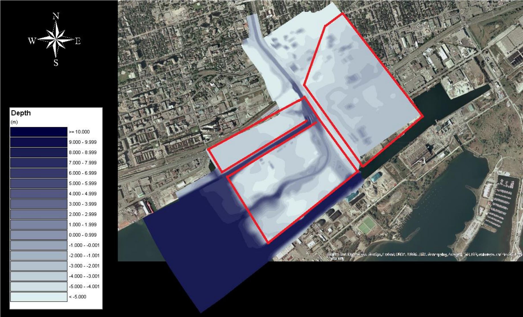
Figure 5.1 Phase 3 model bathymetry. Areas outlined in red indicate where LiDAR data was superseded by MVVA 2015 Phase 3 Grading Plan
