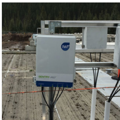
SENTRY, a bio-electrode microbial activity and water quality monitoring platform.
