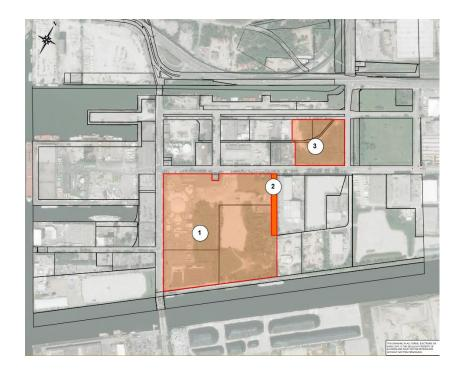
Area 1: Site preparation will include demolition of a parking lot and building as well as clearing of vegetation. Tree cutting in this area is scheduled for August 2018. During tree cutting, we will work with Toronto and Region Conservation to ensure birds and bats are protected.
