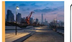
Proposed Pedestrian Lighting Fixture/Pole: Olivio Grande, Asymmetric, 2G350 LED Engine, 3000K CCT Minimum Height: 4.5m Spacing: 15m o.c. Avg. Illuminance: 1.04
