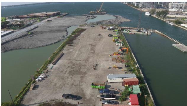
The latest aerial image of the Cherry Street Lakefilling project, showing the new shoreline taking shape, lakefilling progress on the south side of Essroc Quay and dockwall progress to the north.
