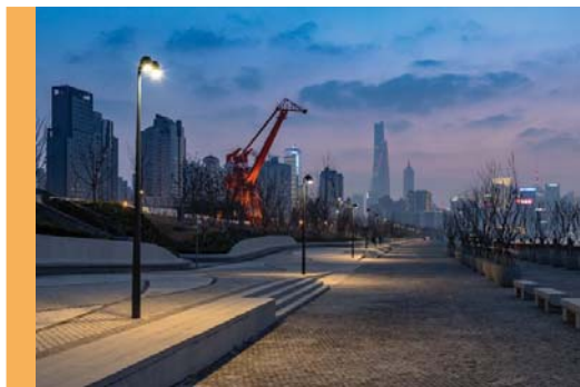
Proposed Pedestrian Lighting Fixture/Pole: Olivia Grande, Asymmetric, 2G350 LED Engine, 3000K CCT Minimum Height: 4.5m Spacing: 15m o.c. Avg. Illuminance: 1.04
