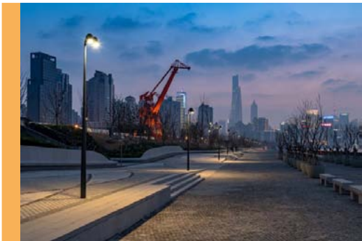
Proposed Pedestrian Lighting Fixture/Pole: Olivio Grande, Asymmetric, 2G350 LED Engine, 3000K CCT Minimum Height: 4.5m Spacing: 15m o.c. Avg. Illuminance: 1.04
