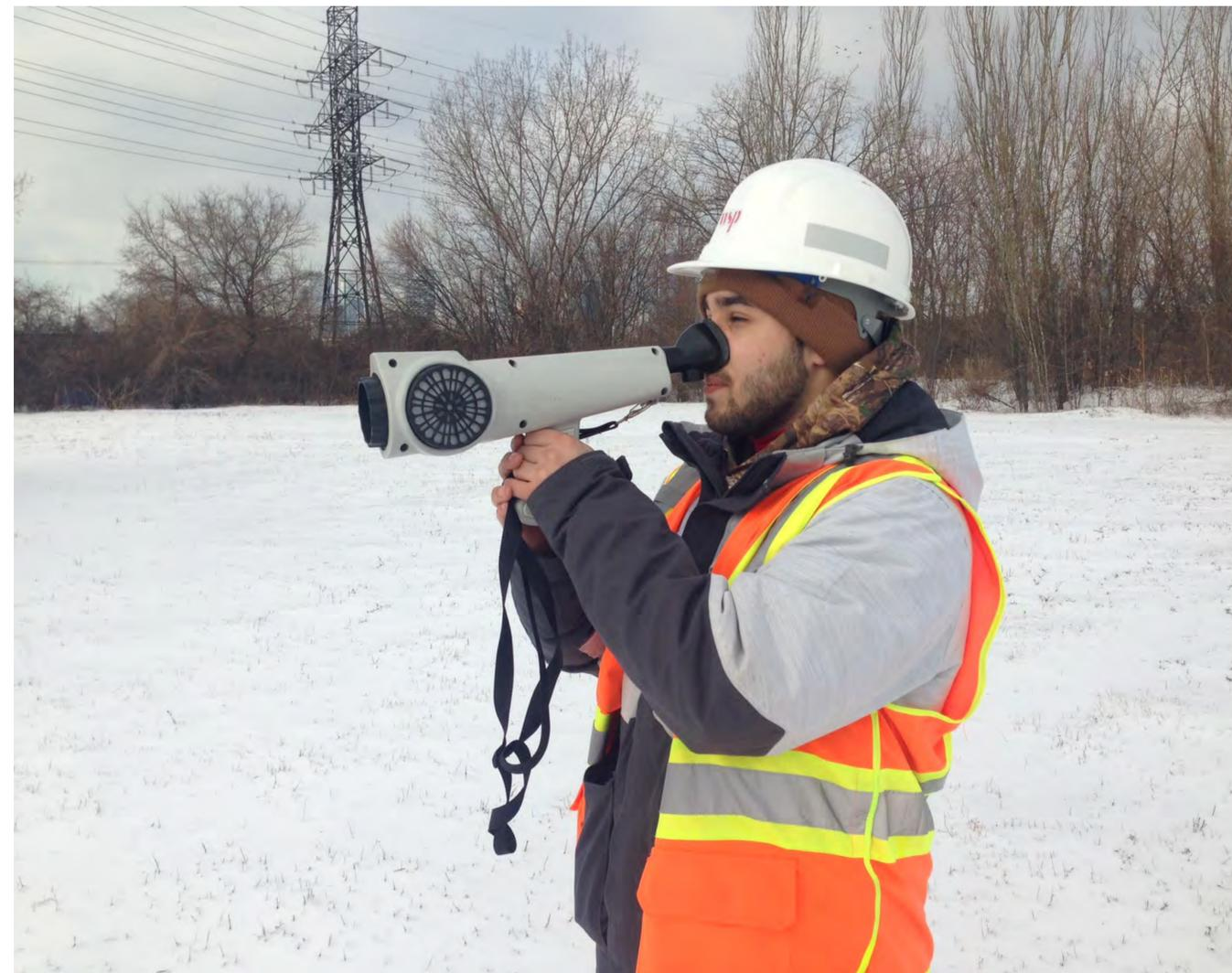
We use a nasal ranger or olfactometer to measure existing odour in and around the construction site.
