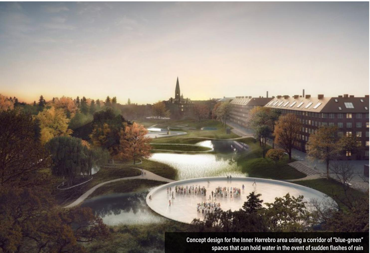
Concept design for the Inner Hørrebro area using a corridor of "blue-green" spaces that can hold water in the event of sudden flashes of rain
