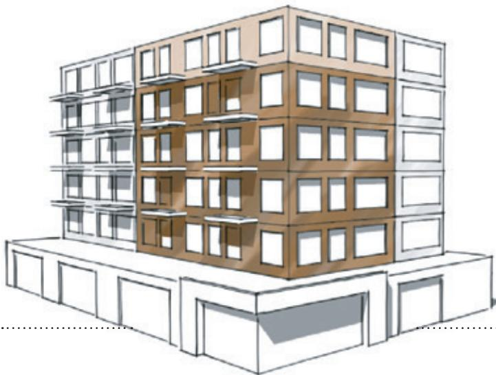
Simple, compact forms for buildings help to minimize thermal bridging through the building envelope.
