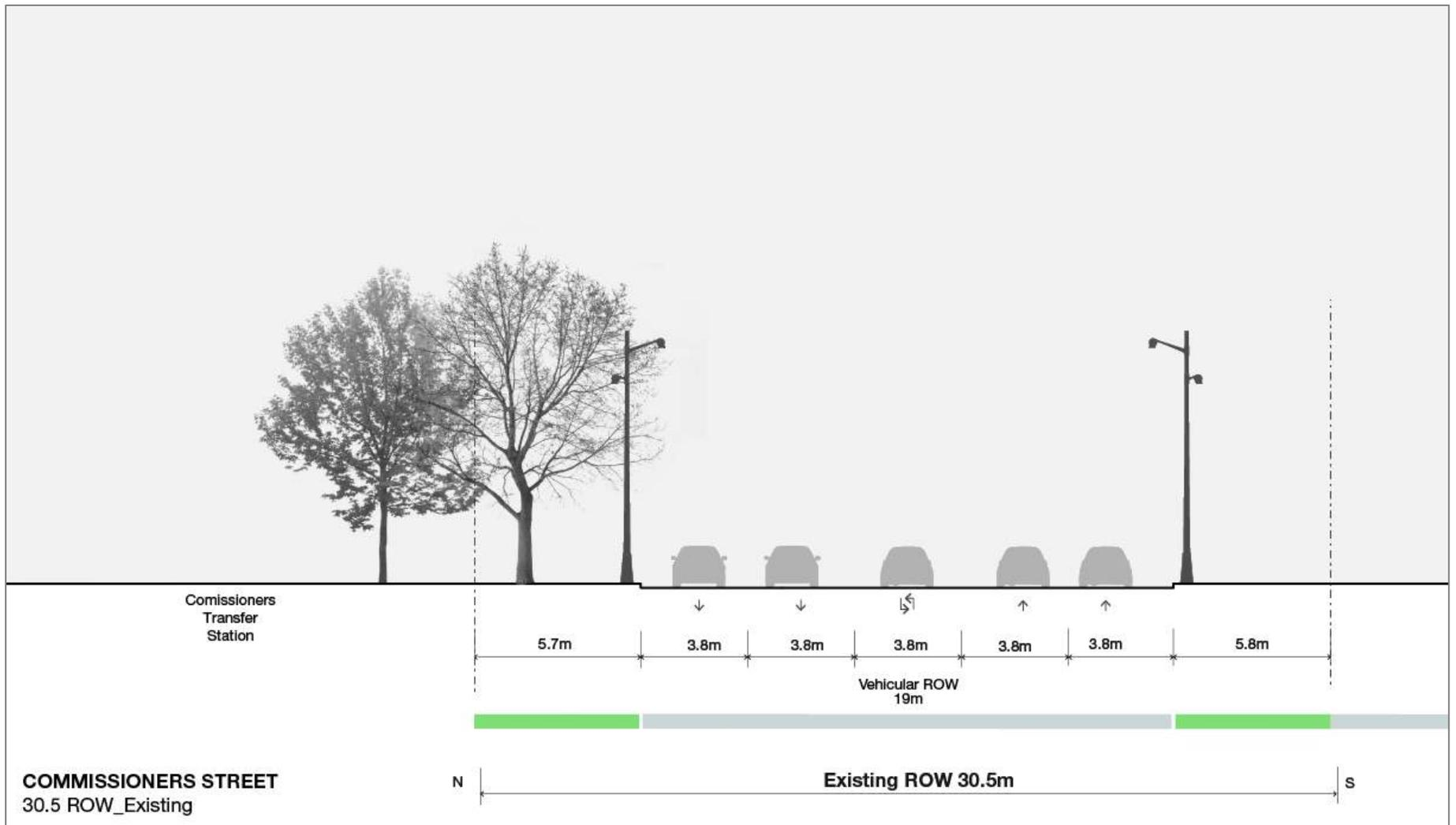
FIGURE 5-35 CROSS-SECTION – EXISTING COMMISSIONERS STREET, ADJACENT TO THE TURNING BASIN
