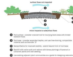
Typical Trail Construction in Wet Soils
