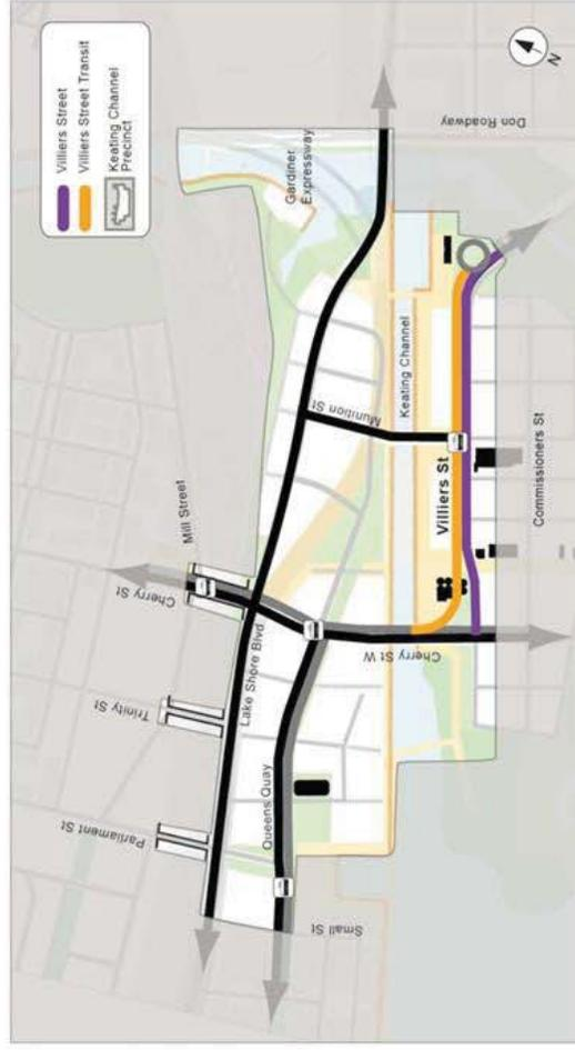
Villiers Street runs east-west within the Keating Channel Precinct. On the north side of the street there are two-way dedicated Light Rail Transit (LRT) lanes. Two lanes of vehicular traffic and one shared turning lane, along with two on-street bicycle lanes are separated from the LRT by a wide, landscaped linear park. For pedestrians there are also 4- to 5-metre sidewalks on both sides of the street.
