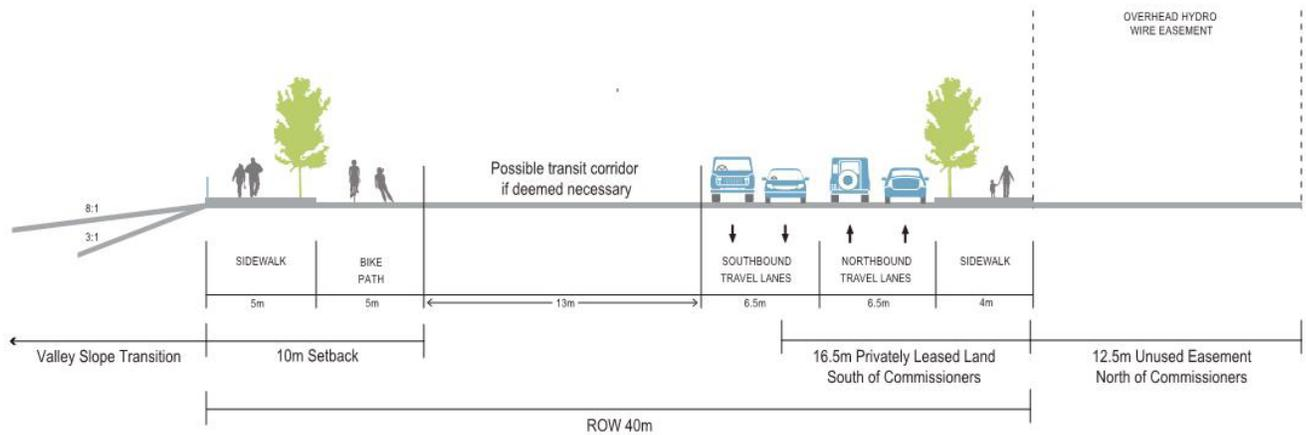
**FIGURE 6-12:** Cross section for Don Roadway between Lake Shore Boulevard East and the ship channel
